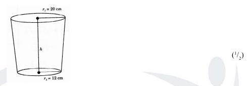
Given: Volume of the frustum is 12308.8 cm<sup>3</sup>. Radii of the top and bottom are R = 20 cm and r = 12 cm, respectively. Volume of the frustum is given by
